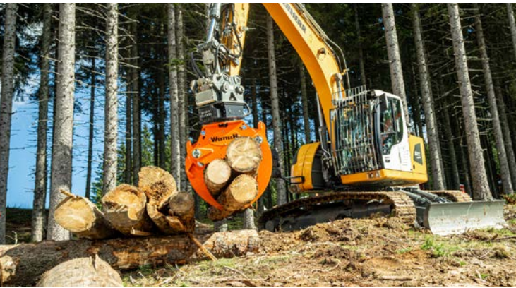
Gripper opening stroke 1270mm.
