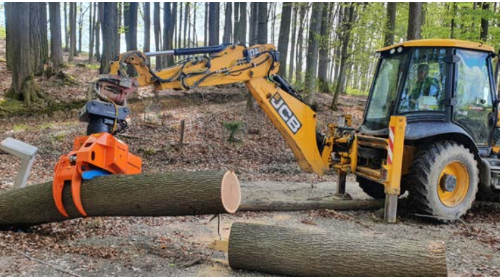
Sturdy and low-wear woodgripper with saw unit.
