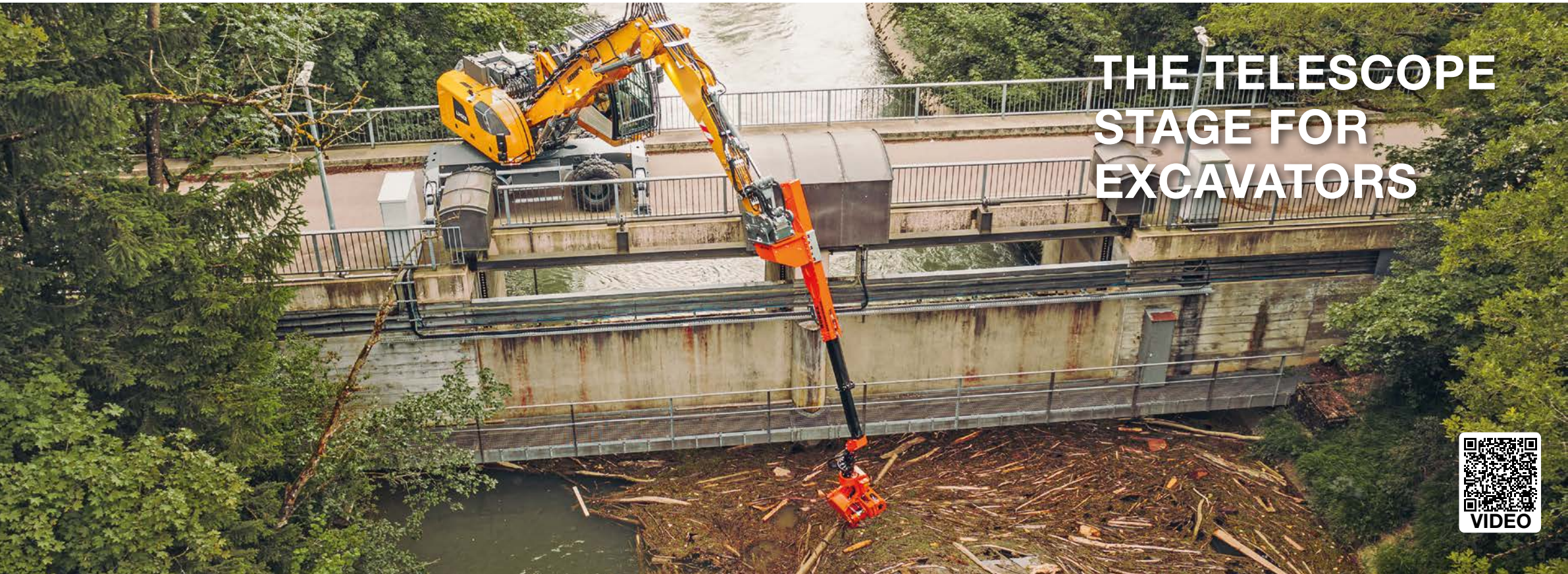
Work range extension up to 6,35 m.
