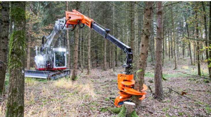
Work range extension up to 6,35 m.
