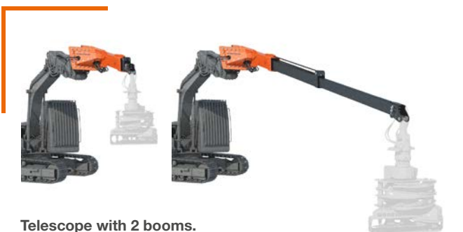
Telescope with 2 booms.
