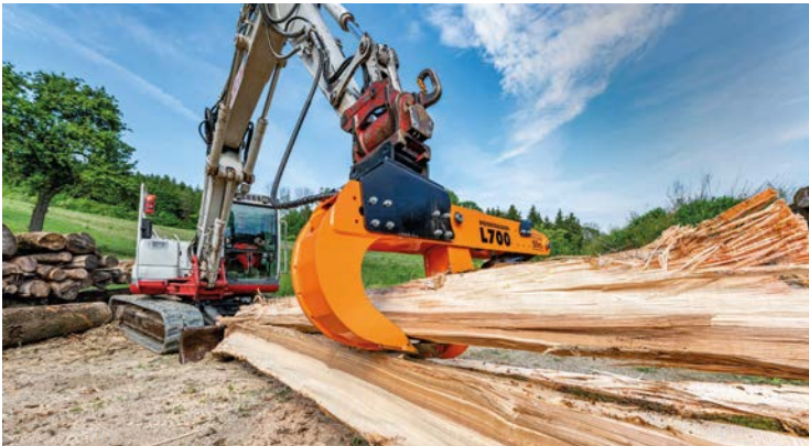
The trunk can be split and loaded in one work step.
